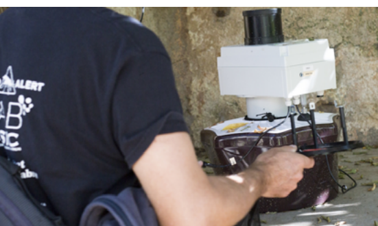
Mosquito trap connected to MIA, one of the information sources used by the EO service.
